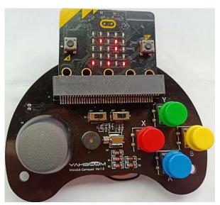
Next, we need to press the B1 button on both handles to start the game, we need to move the red dot by the rocker moving left and right to change the position of the red dot (bullet) below. Press the B3 to launch the red dot(bullet) to the LED dot matrix of the other handle.
